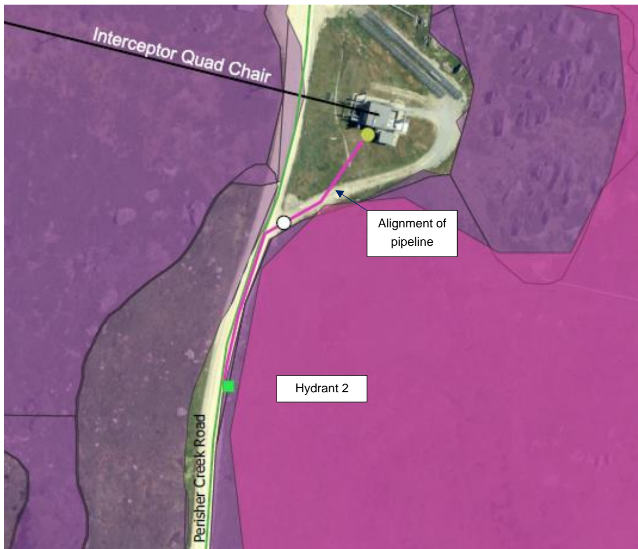
Figure 5 | Alignment of proposal, with hydrant 2 partly within a BVM area (Source: Applicant's documentation)
